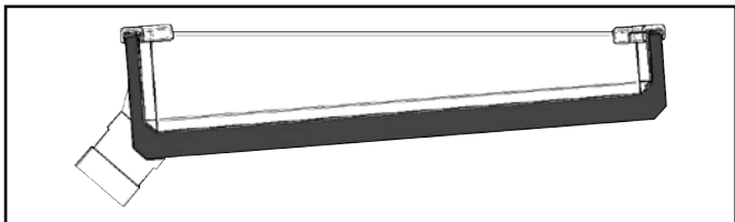
Figure 2 - Sloped Drain Pan
