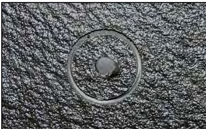
Figure 52 – Scored TripleGuard Corrosion Protection System
